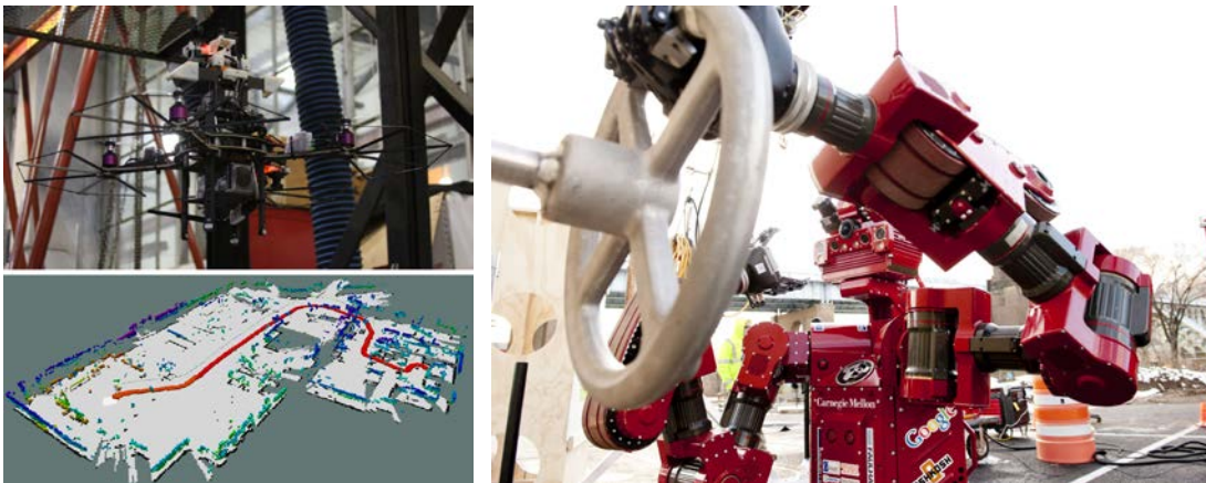
Figure 1: (left) CMU's autonomous MAVs enable mapping and exploration of hazardous indoor environments. (right) CMU's CHIMP turns a valve while operating semi-autonomously at the DARPA Robotics Challenge.
